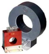
The CBCT or the Core Balance Current Transformer is a current transformer is used for earth fault protection in grounded three phase systems. It is also known as the zero-sequence current transformer. The CBCT is a current transformer through all the three phases are made to pass as in the diagram. Thus the magnetic fluxes caused by the three phase currents cancel each other.
